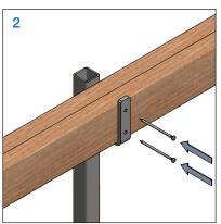
When all the steps are completed, the Parapet Post is ready for the Speed Fence or temporary guardrail to be installed Maximum spacing of Parapet Posts not to exceed 9' (2743 mm)
