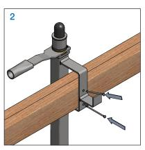
When all the steps are completed, the Slab Grab is ready for the Speed Fence or temporary guardrail to be installed Maximum spacing of Slab Grab not to exceed 9' (2743 mm)
