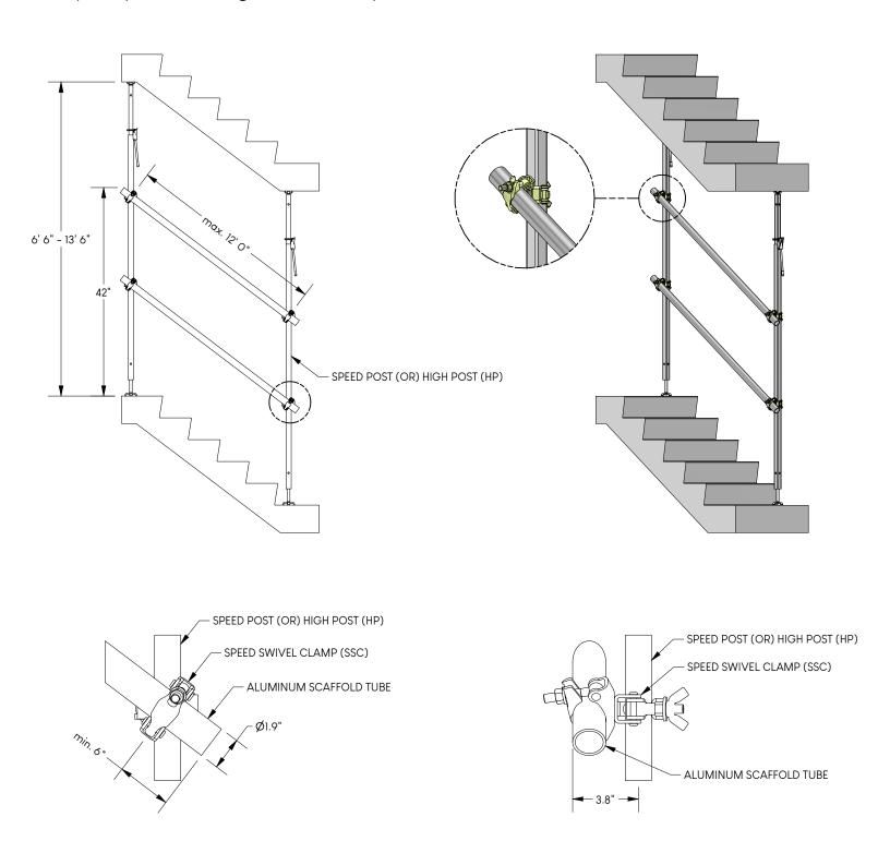
Compliant with all OSHA & Cal/OSHA load requirements for Construction Projects. Maximum span indicated only applies when the guardrail supports are Speed Edge products. Please inquire regarding compliance in other jurisdictions or for special case scenarios. Refer to manual for complete installation instructions.
