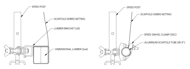
OPTION TO USE LUMBER BRACKET (LB) WITH DIMENSIONAL LUMBER RAILS OR SPEED SWIVEL CLAMP (SSC) WITH SCAFFOLD TUBING
